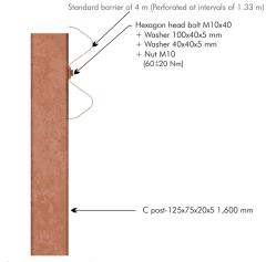
Detail of joint in intermediate post
