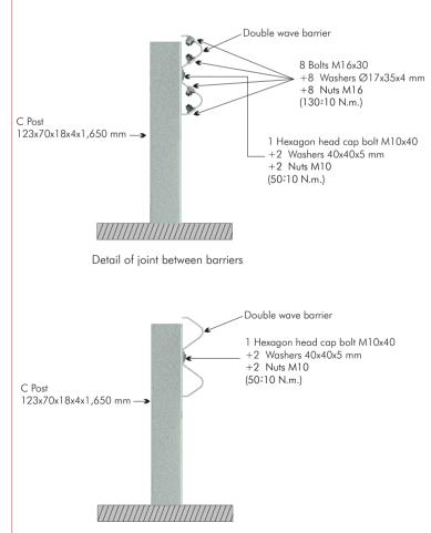
Detail of joint in intermediate post
