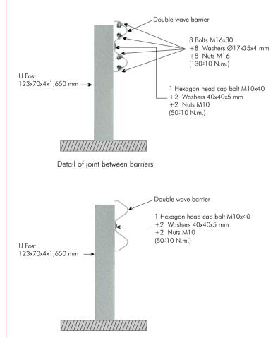
Detail of joint in intermediate post
