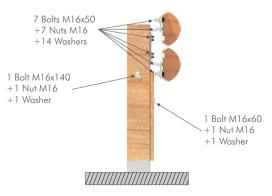
Detail of joint in intermediate post
