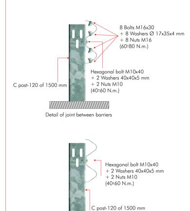
Detail of joint in intermediate post
